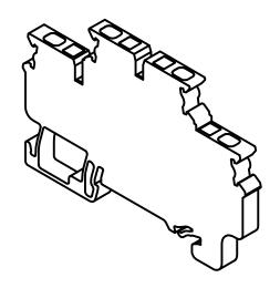
Height with DIN Rail 35 x 7.5 mm 49.5 mm 35 x 15 mm 57 mm
