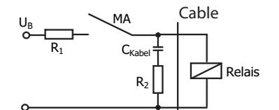
Contact protection with resistors for limiting current
