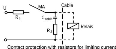
Contact protection with resistors for limiting current
