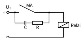
Suppression of voltage peaks with an RC element
